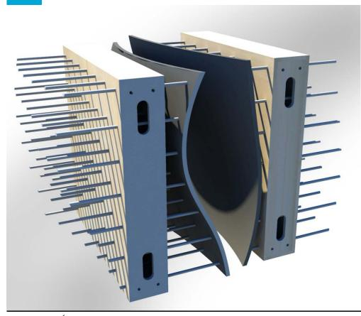
Adding a second adjustable mold allows a void to be formed
