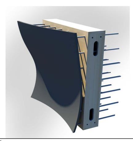
A flexible surface attached to rods that can be moved separately to form doubled curved surfaces
