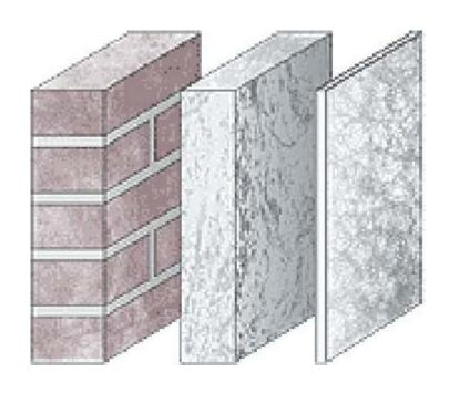
A Phase Change Material is able to store and release heat by a phase change of the material. During the melting process, a lot of heat is absorbed, without raising the temperature of the material.
